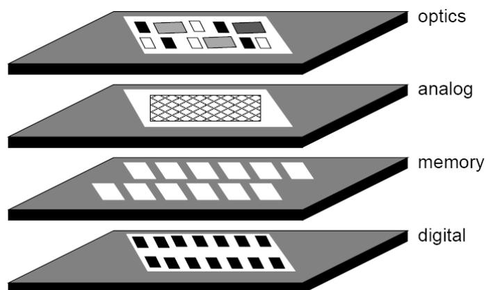
**Figure 7 Principle of 3D heterogeneous integration**
