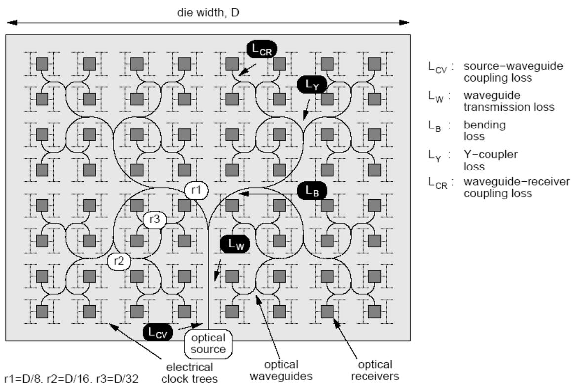
**Figure 15 Possible structure for optical clock distribution network**
