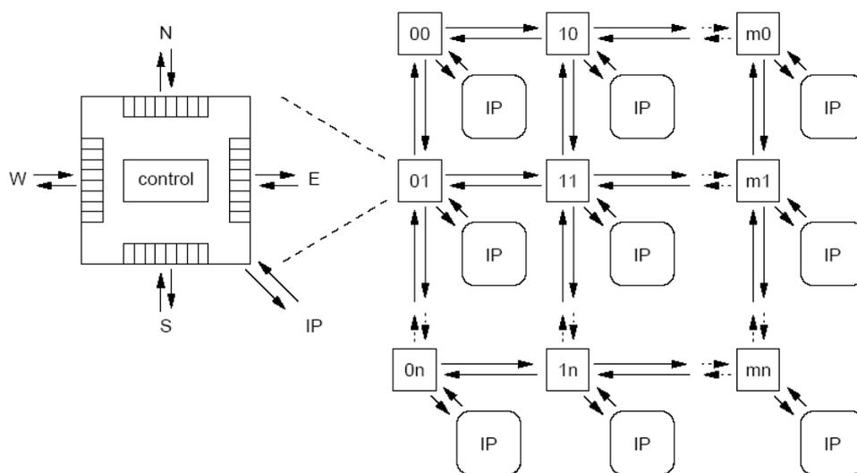
**Figure 12 General NoC architecture showing IP blocks and interconnected switchboxes**
