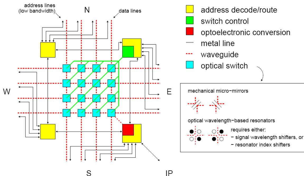
**Figure 13 Switchbox architecture exploiting partial optoelectronic conversion**
