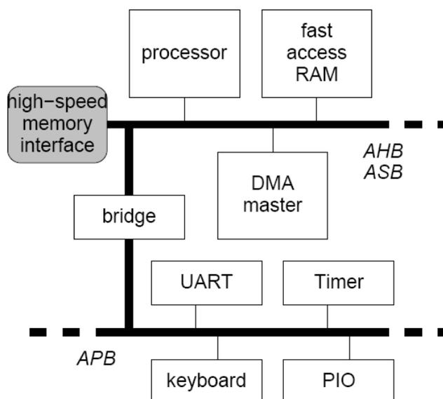
**Figure 9** Example of interconnection by AMBA bus
