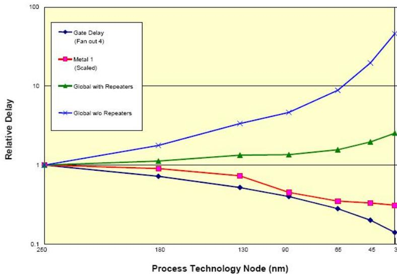
**Figure 2 Gate and wire scaling**
