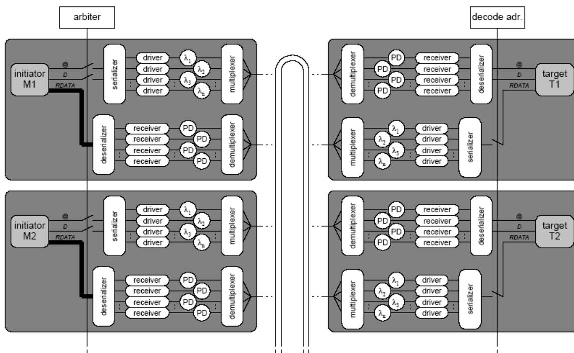
**Figure 11 Possible optical bus structure using TDM and WDM**
