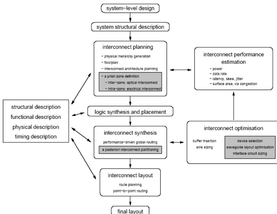
**Figure 16 Interconnect-centric design flow with electrical/optical interconnect partitioning**
