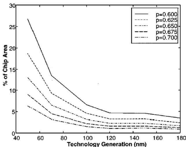
**Figure 8 Silicon area percentage required by interconnect repeaters at different technology nodes**
