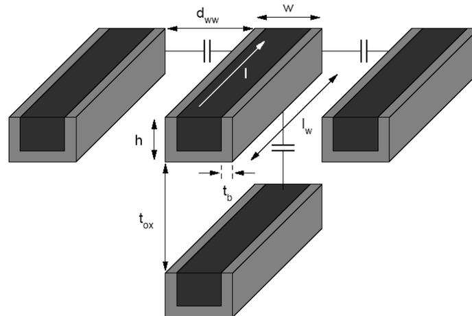
**Figure 3 Definition of interconnect dimensions**
