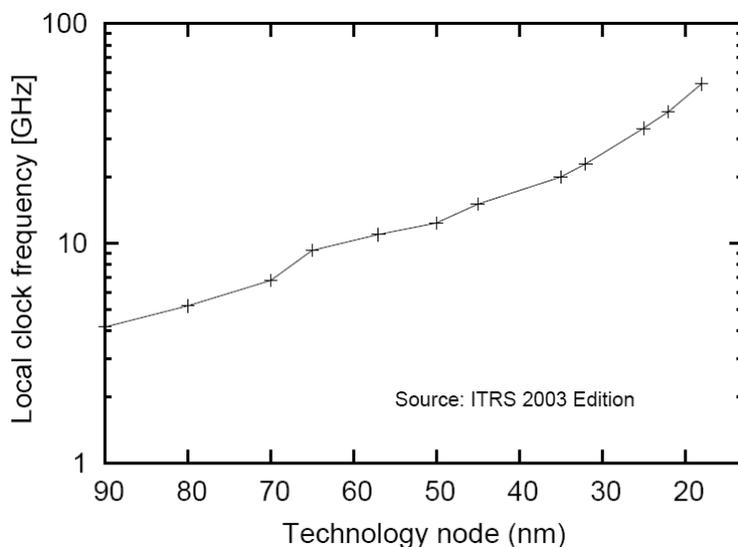
**Figure 1 Progression of local clock frequency with technology node**
