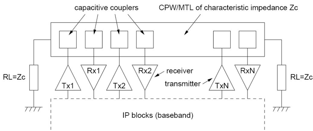
**Figure 6 Integrated RF interconnect channel concept**
