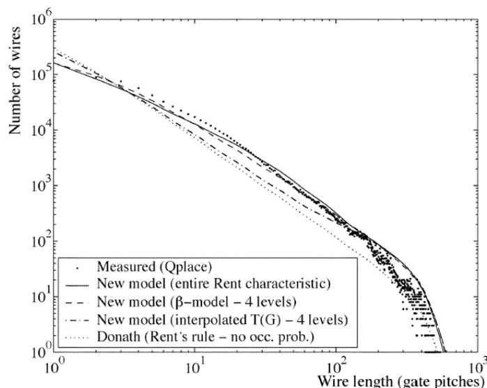
**Figure 4 Interconnect length distribution in a typical processor<sup>6</sup>**
