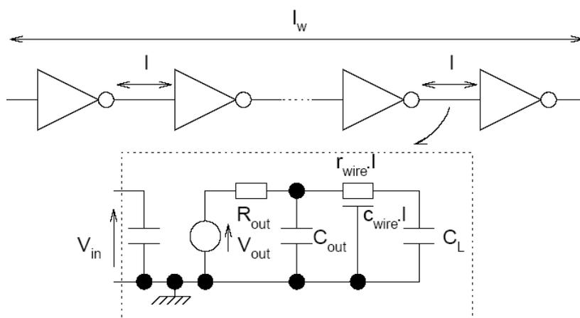
Figure 5 Repeater chain and equivalent circuit
