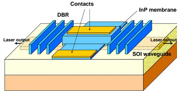
**Figure 2** General layout of the membrane DBR-microlaser
