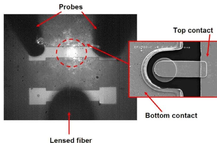
Figure 10 Microdisk laser under test
