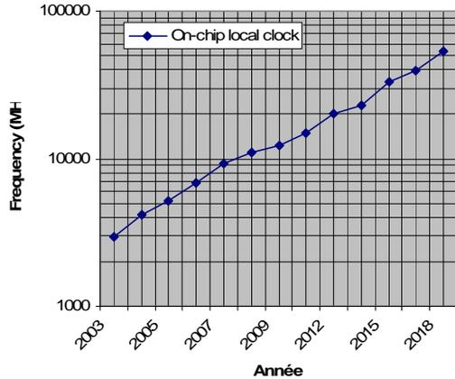
**Figure 11** On-chip local clock frequency predicted by 2003 ITRS
