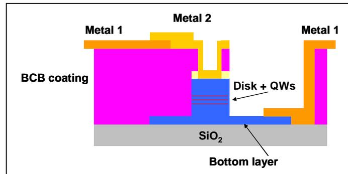
Figure 9 Microdisk source fabrication
