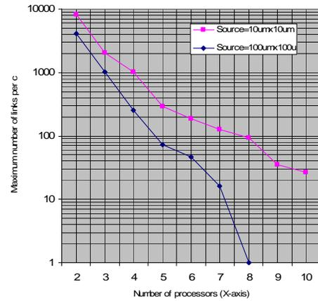
**Figure 12** Maximum number of links per optical channel with respect to number of IP blocks to interconnect and source size
