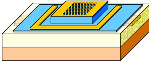
**Figure 5** Electrical injection schemes for the two-dimensional photonic crystal (2DPC) microlaser
