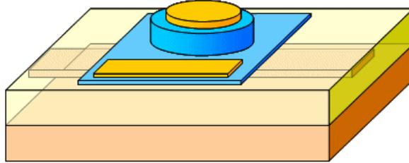
**Figure 8** *Microdisk laser design*
