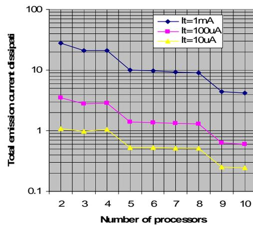
**Figure 14** Total current dissipation in emitter circuits for varying number of interconnected IP blocks (one row only) and source threshold current
