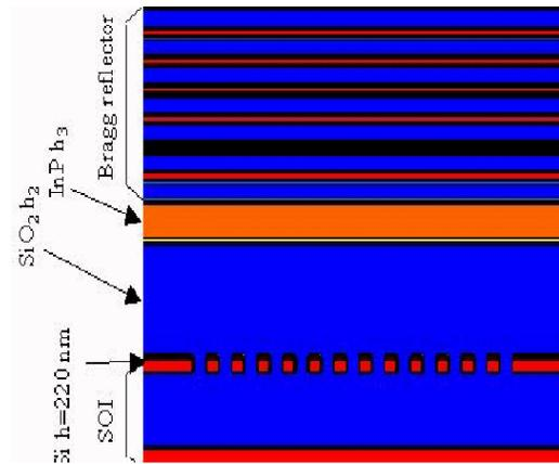
**Figure 7** Cross section view of a diffractively coupled microlaser
