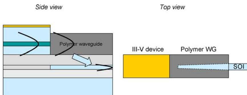
**Figure 1** Design layout of the coupling scheme for semi-compact laser diodes
