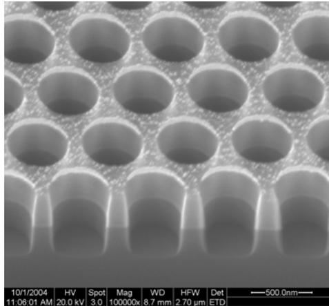
**Figure 6** *Oblique gold evaporation on a photonic crystal pattern*
