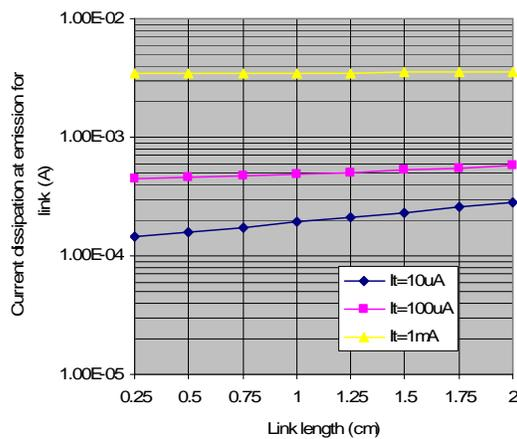
**Figure 13** Current dissipation in emitter circuit (modulator and bias) for varying link lengths and source threshold current
