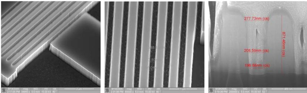
Figure 3 SEM-pictures of DBR structures
