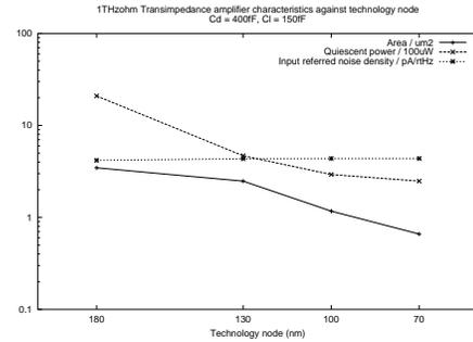
Figure 12: Evolution of TIA characteristics (power, area, noise) with technology node
