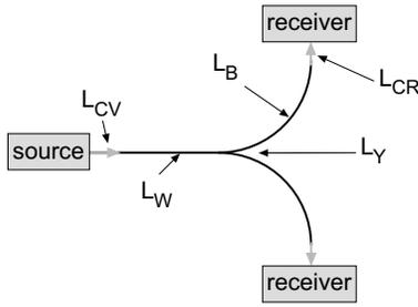
Figure 3: Losses in an optical link
