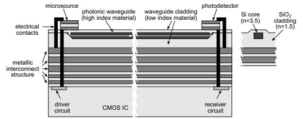
Figure 2: Cross-section of hybridised interconnection structure
