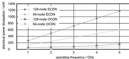
**Figure 18: Electrical power dissipated by electrical (ECDN) and optical (OCDN) clock distribution networks for varying operating frequency**
