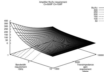
Figure 11: TIA  $R_o/A_v$  design space with varying bandwidth and transimpedance gain requirements
