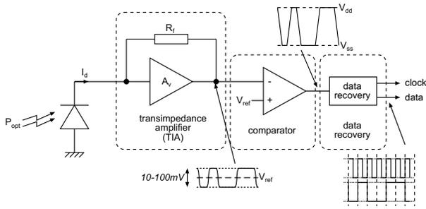
Figure 9: Typical photoreceiver circuit
