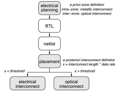
**Figure 14: Design flow modifications for integrated optical interconnect**
