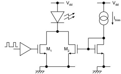
**Figure 8: Basic current modulation source driver circuit**
