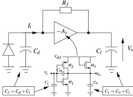
Figure 10: CMOS transimpedance amplifier structure
