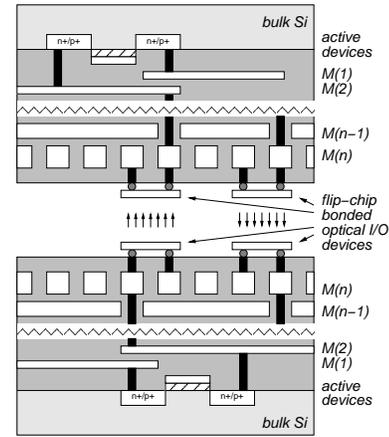
**Figure 1: Inter-chip communication using flip-chip bonded optical I/O devices**
