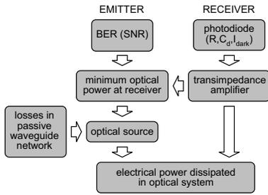
**Figure 13: Methodology used to estimate the electrical power dissipation in an optical clock distribution network**
