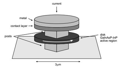
**Figure 7: Structure of a microdisk laser**
