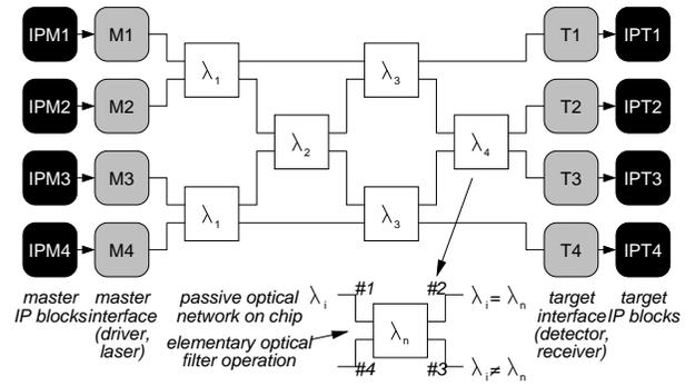
**Figure 19: Architecture of 4x4 optical network on chip**
