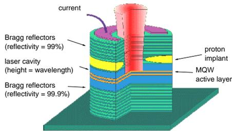
**Figure 6: Vertical cavity surface emitting laser (VCSEL) structure**
