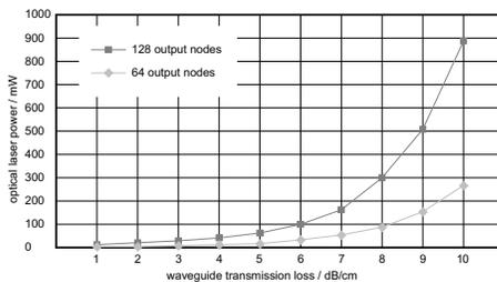
**Figure 17: VCSEL optical output power required by the H-tree to provide a given BER for varying waveguide transmission loss**
