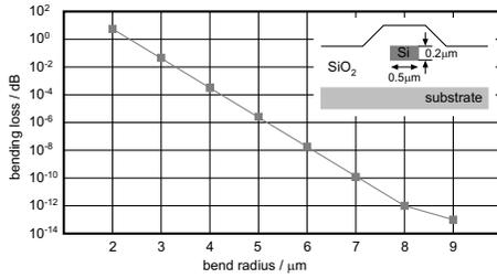
Figure 4: Simulated bending loss for Si/SiO<sub>2</sub> strip waveguide
