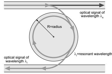
Figure 5: Micro-disk realisation of an add-drop filter
