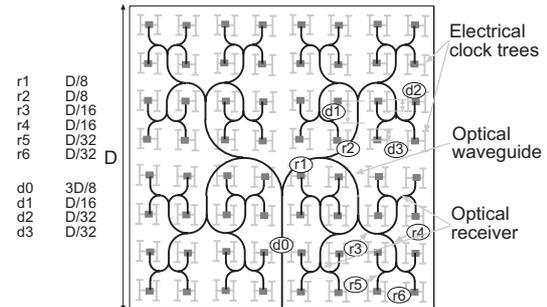
**Figure 5. Optical H-tree network with 64 output nodes.**
