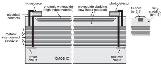
**Figure 4. Cross section of hybridised interconnection structure**
