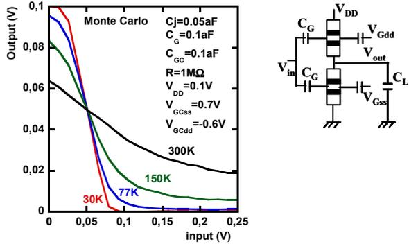
**Figure 9: transfer characteristics of a SET inverter**
