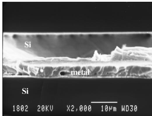
Figure 4: Cross section of Si to Si bonded dies.
