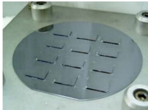
Figure 5. Four-inch Si wafer with multiple dies bonded on specific regions
